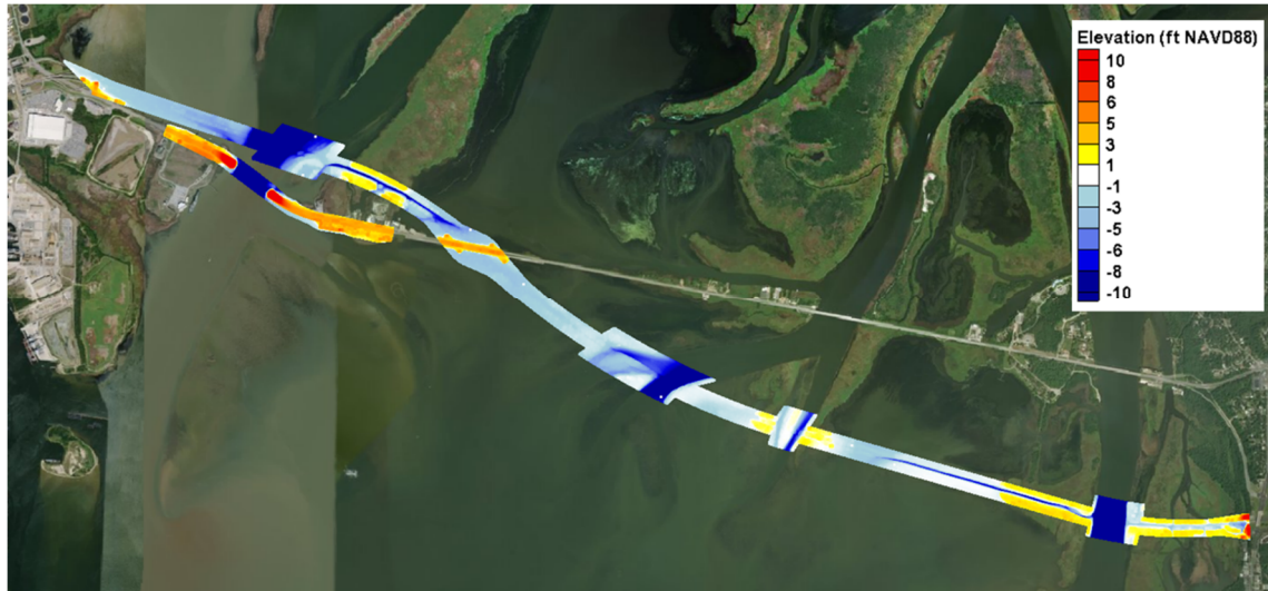
Figure 2. Bathymetry and Topography data collected for ALDOT (Tremble, 2017)
